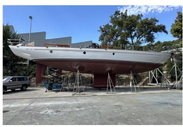
This very special "in-build" sailing yacht is a true world cruiser, constructed entirely from Duplex Stainless-Steel (SAF 2205- Duplex). To be rigged as a ketch, she is set up for short-handed cruising in style, comfort and safety.
